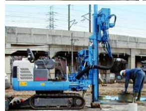
Extracting a sample with a simple boring machine
